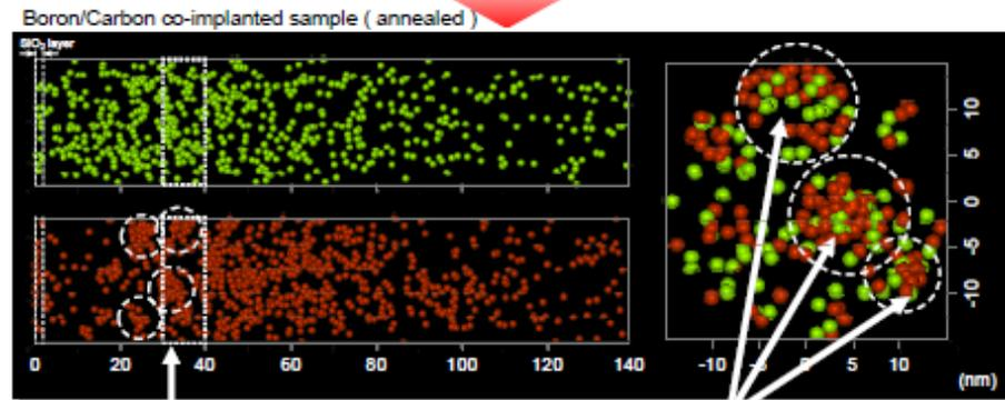
Depth of co-clusters obtained by APT is consistent with that at the locally-high concentration of boron and carbon by SIMS
